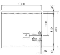
Gas Gas Power: 41 kW Gas Type Option: Gas Inlet: 1/2" **Key Information:** Oven working Temperature: 80 °C MIN; 300 °C MAX Oven Cavity Dimensions (width): 683 mm **Oven Cavity Dimensions** 255 mm (height): Oven Cavity Dimensions 671 mm (depth): External dimensions, Width: 1000 mm External dimensions, Depth: 900 mm External dimensions, Height: 700 mm Net weight: 173 kg Both-Sides Operated;On Configuration: Oven Front Burners Power: 8.5 - 8.5 kW **Back Burners Power:** 8.5 - 8.5 kW
